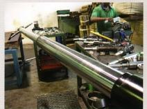
Every tube section precision supported by the super smooth guide ring. Good concentricity between sections are maintained throughout the stroke movement.
