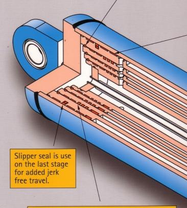
Special precision ground finish carbon composite piston seal rings are used in our cylinder. They are able to create a jerk free movement. The fact that they are specially ground to a unique profile that offers good sealing and jam free passage.
